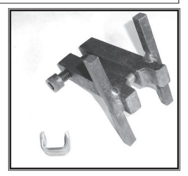
I've made 20 or more trivets like this for gifts and as a result have a whole set of jigs to speed up the process. I've always fought the collars, so I recently made this collaring jig. Now I can install three collars in about 5 minutes.
